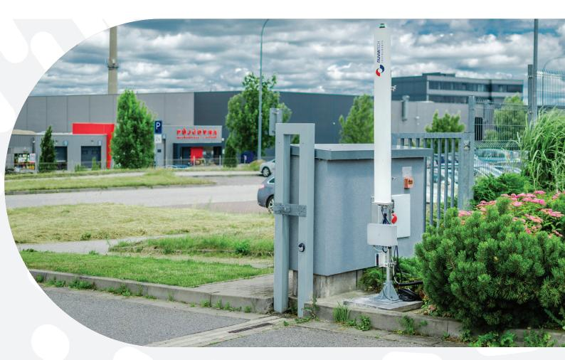
The NuCLEARANCE Lite is equipped with two 5L scintillation detector, designed for quick and easy inspection of vehicles transporting scrap metal. The high sensitivity of the detection system guarantees high reliability of detection of potential sources of ionizing radiation for a minimal investment.
