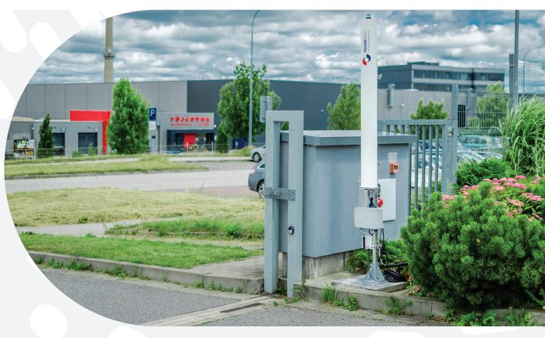
The NuCLEARANCE Lite is equipped with two 5L scintillation detector, designed for quick and easy inspection of vehicles transporting scrap metal. The high sensitivity of the detection system guarantees high reliability of detection of potential sources of ionizing radiation for a minimal investment.
