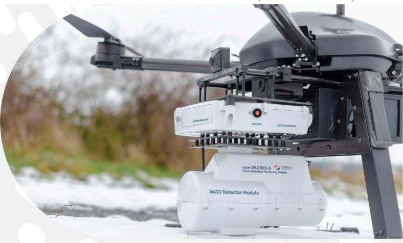
NUVIATech delivers a fully integrated aerial radiation monitoring solution, combining a high-performance UAV with advanced DRONES-G modules. Designed for airborne radiation surveys, emergency response, and environmental monitoring, this system ensures real-time, high-precision radiation detection and mapping. Unlike standard UAVs, it provides a complete, turnkey solution with seamless integration of specialized measurement technology.
